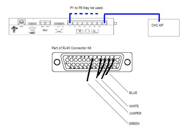
The CHC appears to require wiring as if it were a DTE device. As the FieldServer is A DTE device this implies the cable is NULL Modem Like.
